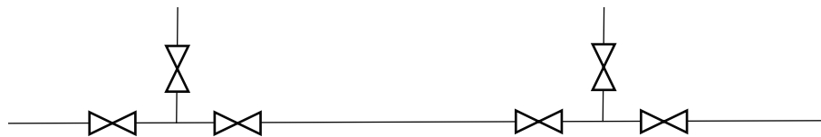
Typical ring valved take off points to two departments
